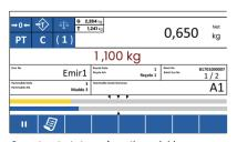
Operator starts to perform the weighing process with the help of both weight and bar graph
